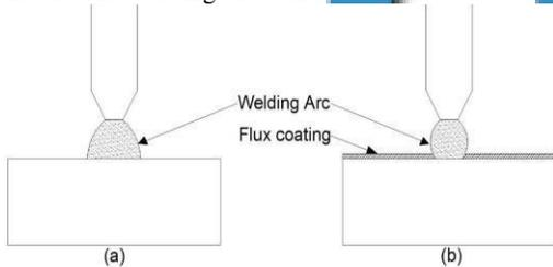
Figure : Schematics of the welding arc in (a) TIG welding, and (b) FCTIG welding.
